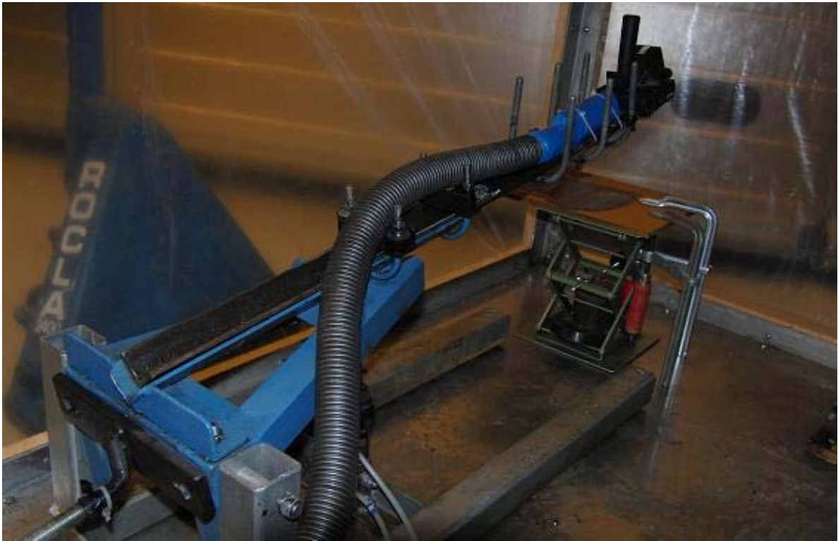
Figure 2.4 MBX Bristle Blaster mounted inside the test volume prior to testing.
