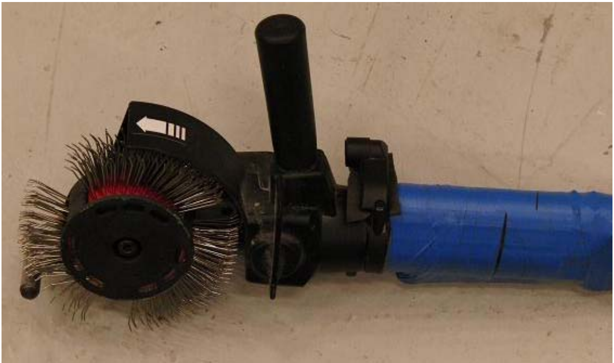
Figure 2.2 Modifications made to the MBX Bristle Blaster in order to test the tool in an explosive atmosphere.
