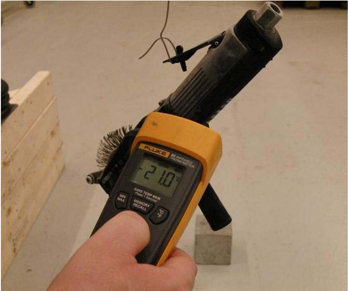
Figure 2.1 Photograph showing the tool hanging in the stand prior to testing. The tool has a temperature of -21 °C.
