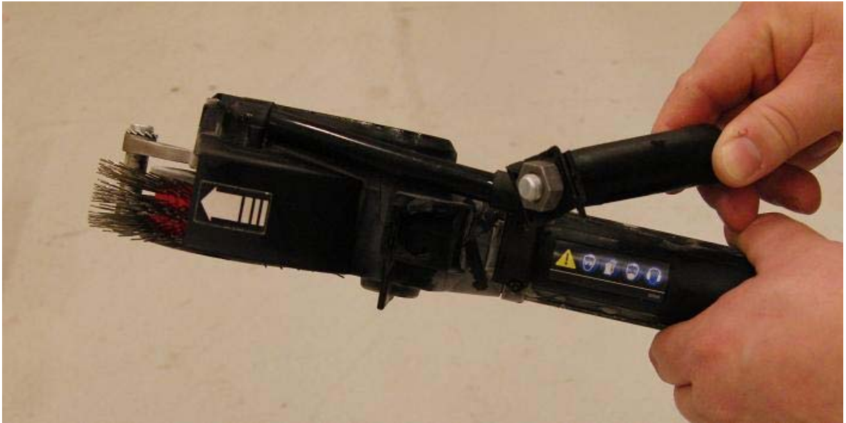
Figure 3.2 Picture showing the damage on the tool after the second drop.
