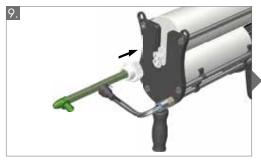
Install spray nozzle onto cartridge and secure with retaining ring by turning 60 deg clockwise.
