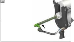
Connect atomizing air line to spray nozzle.
