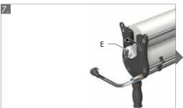
Remove cartridge nose plug (E) by turning retai ning nut 120 deg counterclockwise.
